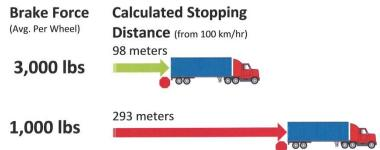
Beyond the DOT readjustment limit, brake force decreases significantly and at the manufacturer's rated travel limit, brake force is virtually non-existent.
