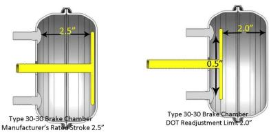
The DOT mandates a readjustment point commencing  $\frac{1/2}{2}$  inch before the manufacturer's rated stroke is reached to ensure that effective braking will occur in both normal and emergency situations.
