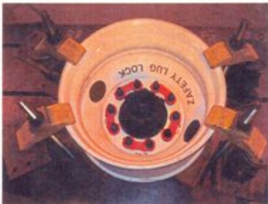
Figure 2 : Test set-up – Samples installed on nuts, steel drum
