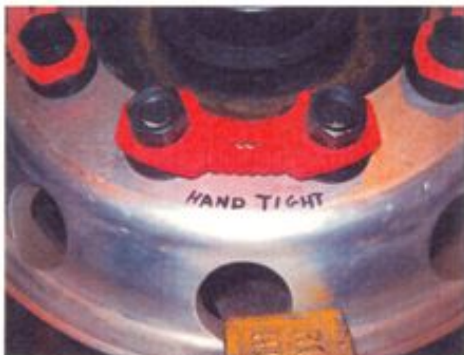
Figure 8 : Sample 10-03-C0152-6 installed on hand tight nuts
