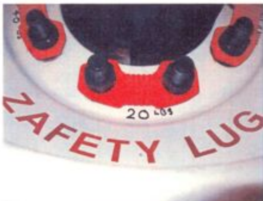
Figure 4 : Sample 10-03-C0152-2 installed on 20 ft-lb torque nuts
