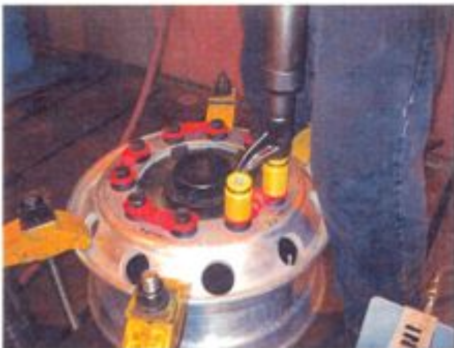
Figure 13 : Example of torque applied with the air gun
