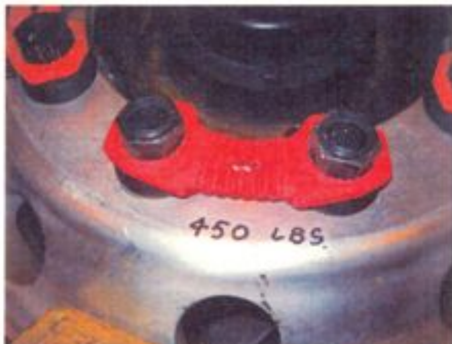
Figure 12 : Sample 10-03-C0152-10 installed on 450 ft-lb torque nuts
