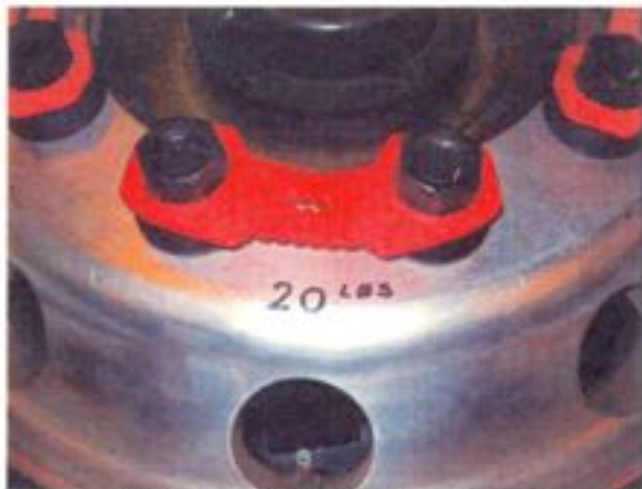
Figure 9 : Sample 10-03-C0152-7 installed on 20 ft-lb torque nuts
