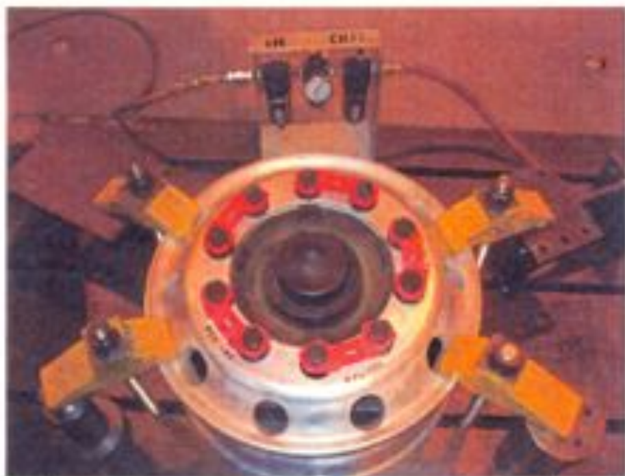
Figure 1 : Test set-up – Samples installed on nuts, aluminium drum
