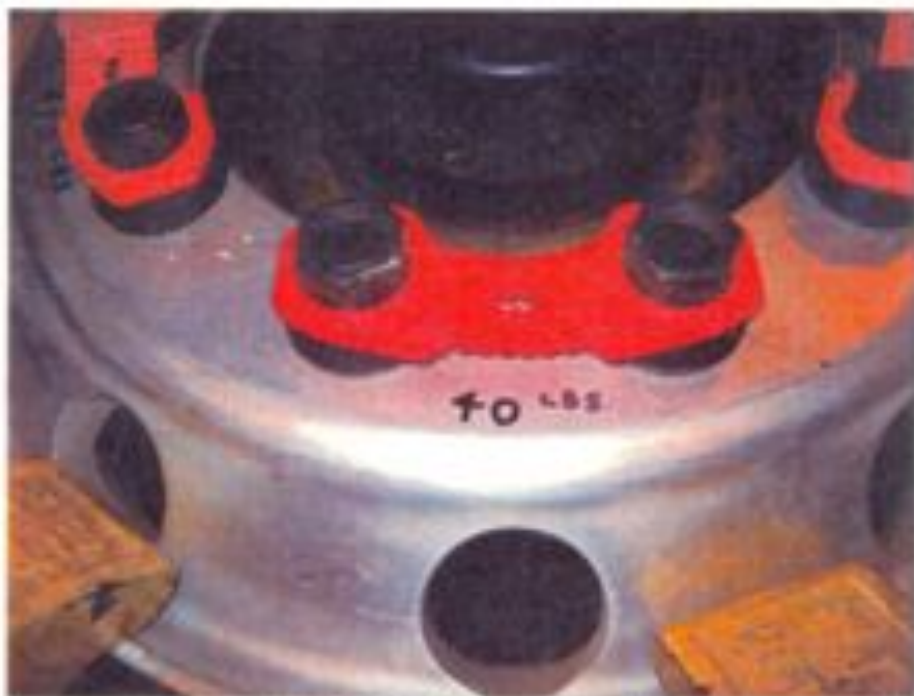
Figure 10 : Sample 10-03-C0152-8 installed on 40 ft-lb torque nuts
