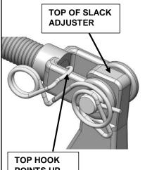
The anti-seize cotter pin kit comes with opposite side cotter pins that can be installed on either side depending on the direction of the slack adjuster (up or down) and the clevis pin hole orientation (left or right).
