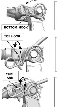
Rotate the pin forward towards the front of the voke such that the bottom hook is positioned underneath the yoke arm.
