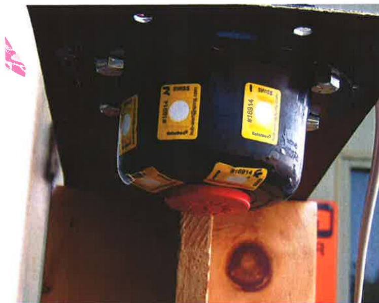
Figure 13A : Temperature activation test set-up for plastic hub cap
