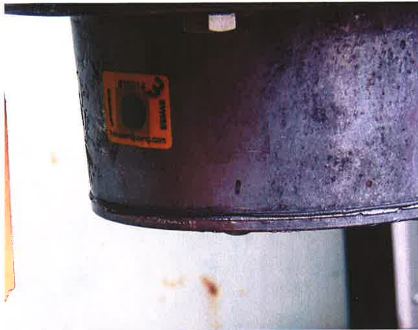
Figure 21A : Aluminum hub cap, showing complete temperature activation of HUB ALERT™ heat sensing label (Exova sample numbers 11-15-0165-40)
