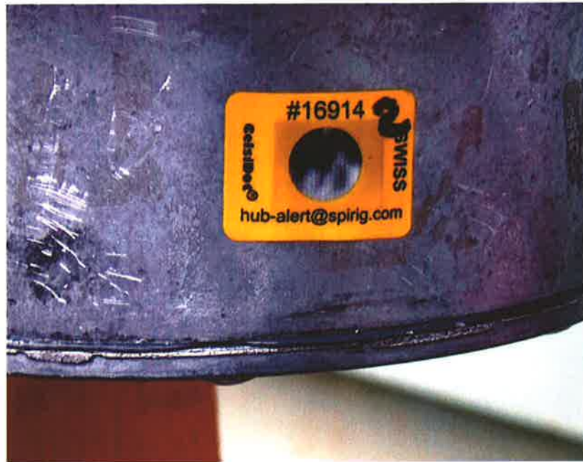
Figure 19A : Aluminum hub cap, showing partial temperature activation of HUB ALERT™ heat sensing label (Exova sample numbers 11-15-0165-39)
