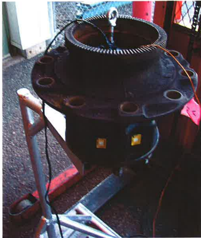
Figure 5A : Temperature activation test set-up for the steel hub and hub cap
