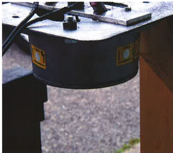
Figure 18A : Temperature activation test set-up for plastic hub cap
