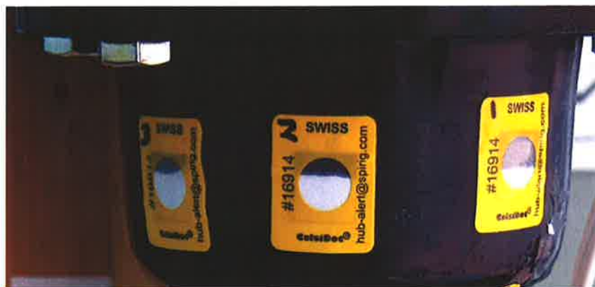
Figure 16A : Plastic hub cap, showing partial temperature activation of HUB ALERT™ heat sensing labels (Exova sample numbers 11-15-0165-33 to 35 labels applied to side of hub cap)
