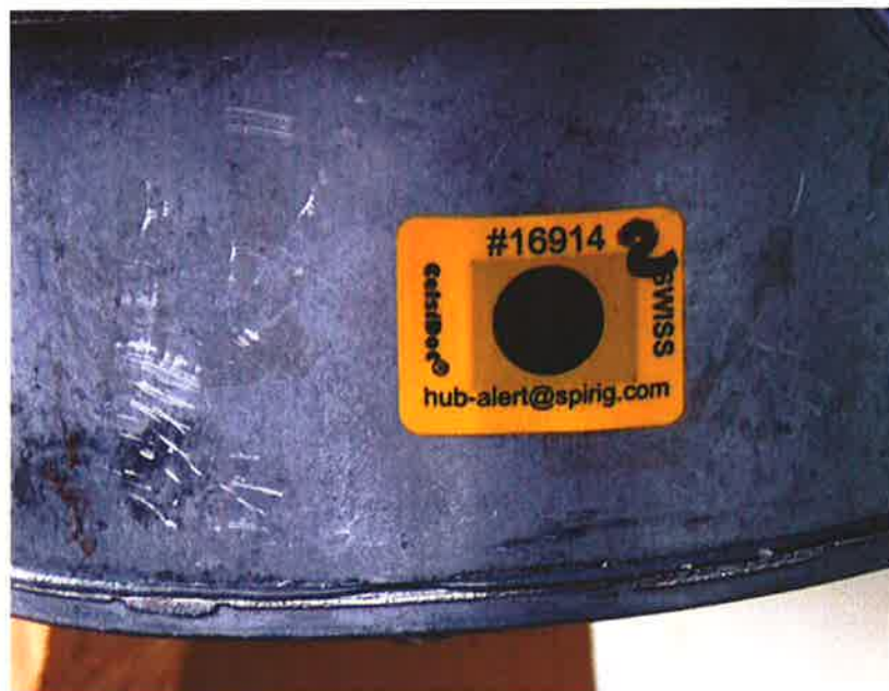
Figure 20A : Aluminum hub cap, showing complete temperature activation of HUB ALERT™ heat sensing label (Exova sample numbers 11-15-0165-39)
