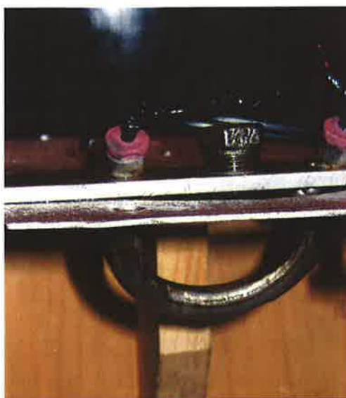
Figure 4A : The heating element for insertion into the oil-filled hub cap (plastic and aluminum hub caps)
