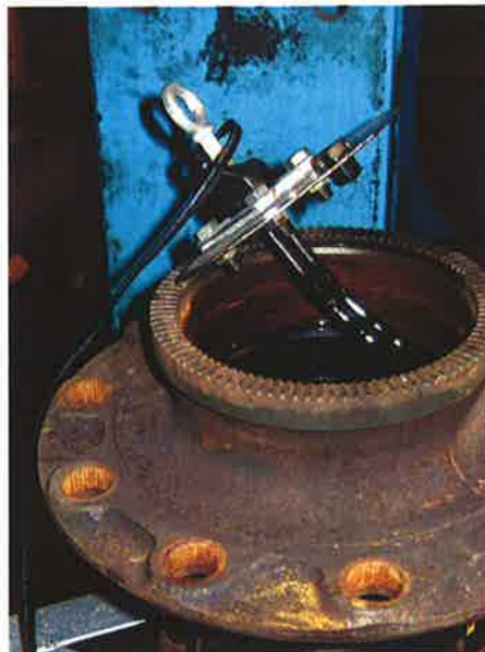
Figure 2A : The heating element for insertion into the oil-filled hub
