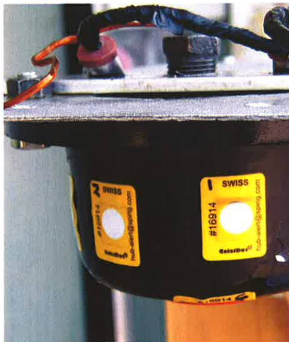
Figure 14A : Plastic hub cap, showing partial temperature activation of HUB ALERT™ heat sensing label (Exova sample numbers 11-15-0165-33, labels applied to side of hub cap)
